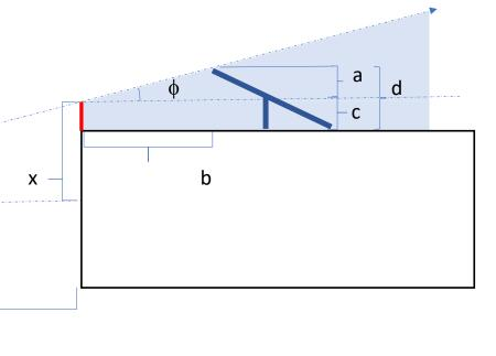
\*Utilizing the shortest height of the parapet considers the worst-case scenario, and therefore allows us to ignore the slope of the roof to establish compliance. If compliance cannot be established under worst-case conditions, applicant can customize these calculations to more accurately reflect distance "c" based on actual site conditions.
